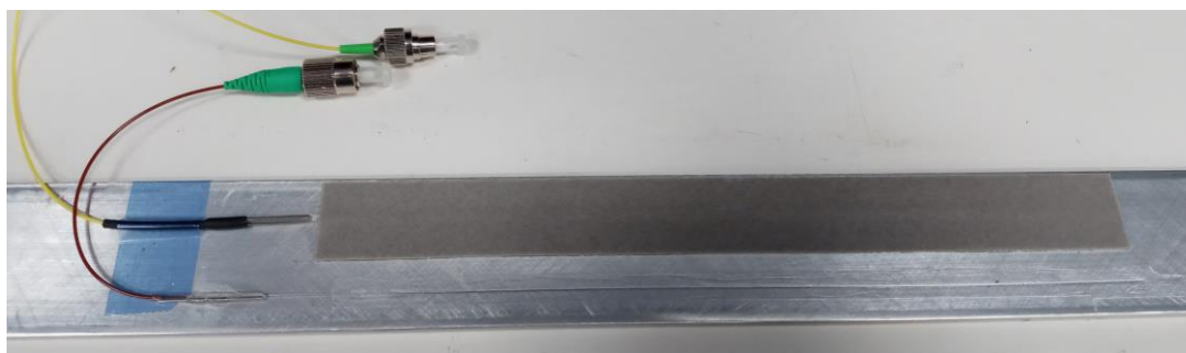
Figure 3. Tape installation and M-Bond 200 installation.
