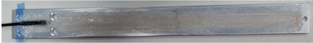
Figure 1. Fiber installed with adhesives can be covered with RTV for environmental protection.
