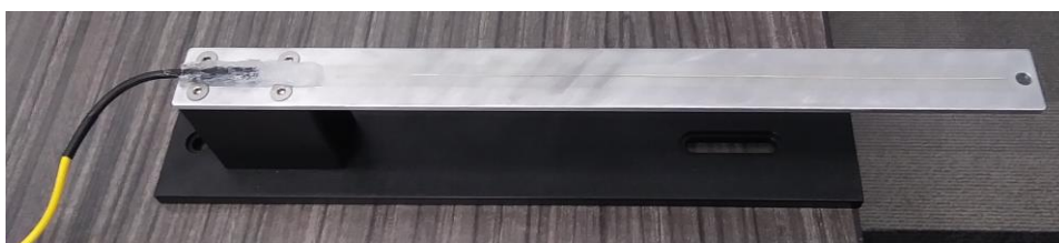
Figure 1. A demonstration cantilever beam with an installed fiber is part of Sensuron's offering included with Strain Sense interrogators to provide users with a simple and effective initial experience.
